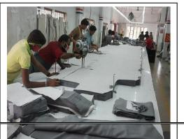
After getting approval to start cutting, cutting staff will open all rolls of fabric required for days cutting at least 24 hours prior to commencement of cutting for the purpose of fabric setting. This fabric setting is required to make the fabric return to its actual shrink form.
